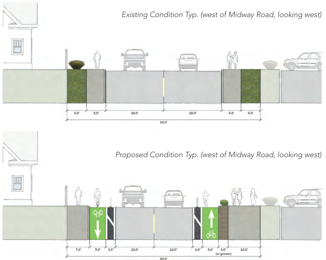
Figure 5-2: Beltway Drive Bike Lanes and Wide Sidewalk
