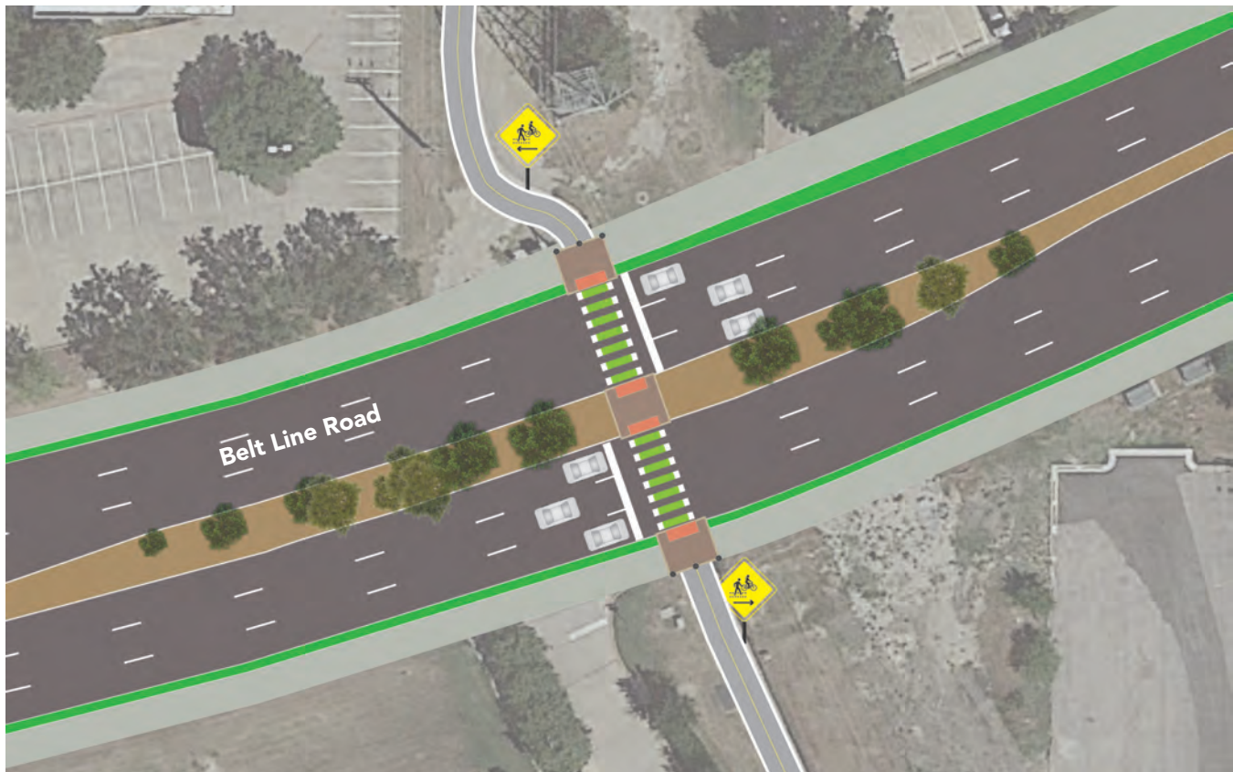
Figure 4-14: Prototypical Arterial Street Mid-Block Crossing (Belt Line Road)
